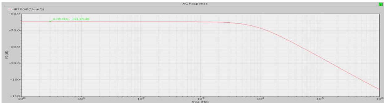
Fig 3.3 AC response of the Op-Amp showing CMRR
