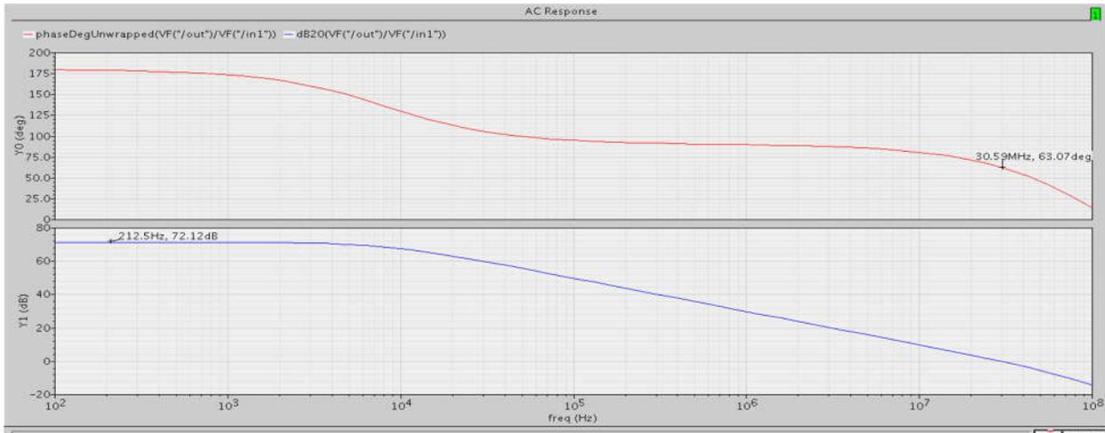
Fig 3.1 Frequency response of the proposed Op-Amp
