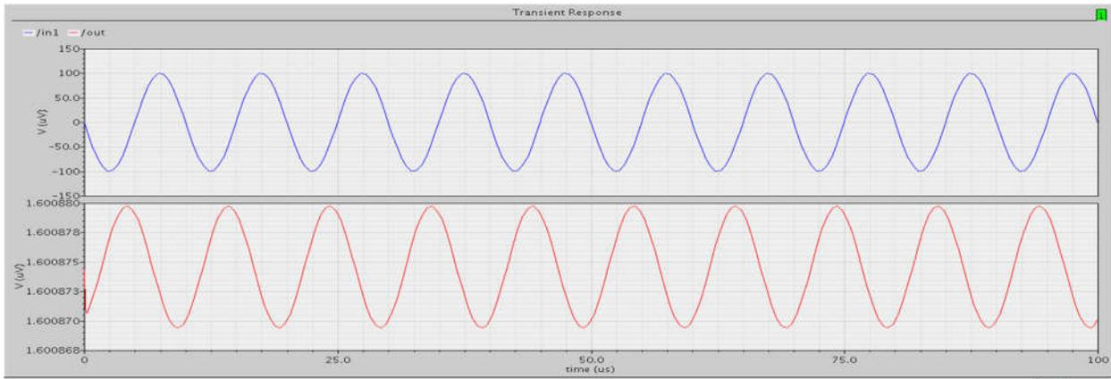
Fig 3.2 Transient Response of the Op-Amp
