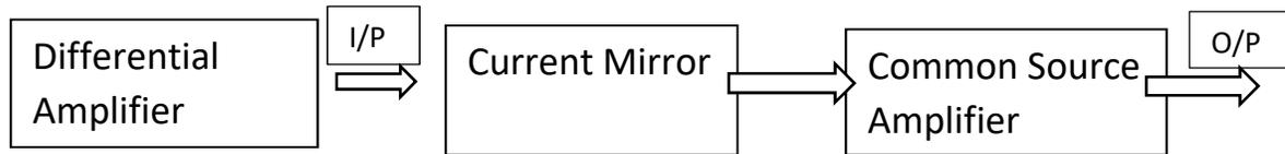
Fig. 2.1 Block Diagram of Proposed Op-Amp
